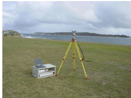
Figure 2. L1 C/A pseudolite physical configuration.
