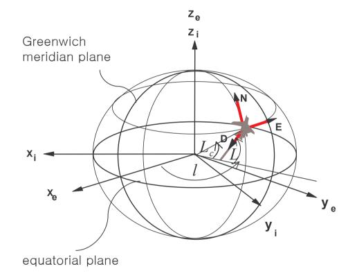
• Locally-Level Frame (n-frame) – The z-axis points toward the interior of the ellipsoid along the ellipsoid normal. The x-axis points toward true north. The y-axis follows the right-handed rule.
