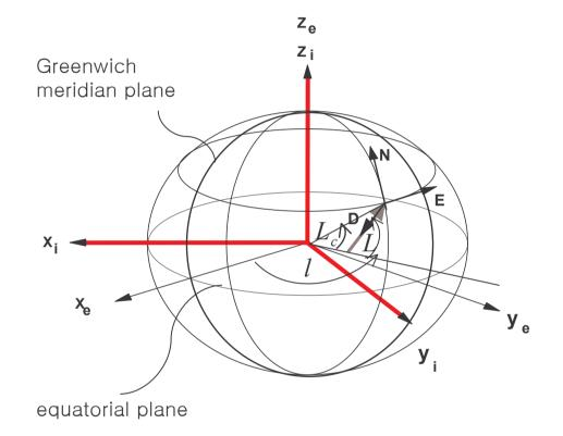
Inertial Frame (i-frame) – A reference frame in which Newton's laws of motion apply. Non-accelerating but may be in uniform linear motion. An orthogonal coordinate system.
