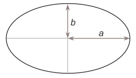
semi-major Axis: a = 6378137 (m)semi-minor Axis: b = 6356752.3142 (m)flatness: f = (a-b)/a = 1/298.257223563 = 0.00335281066475eccentricity:  $e = [f(2-f)]^{1/2} = 0.08181919084262$
